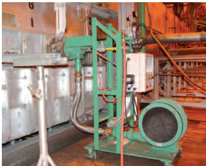
COMPLETE SKID MOUNTED SYSTEM PREPIPED AND PREWIRED FOR PLUG AND PLAY OPERATION ON THE JOB SITE (USING TFB BURNER)
