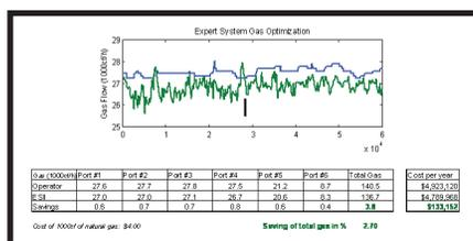
▲ Fig 3. ESIII gas fuel optimisation compared with manual operator's control.
