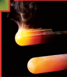
process, corrosion and cost conditions of the glass melting process. Molybdenum has been the standard choice for decades, because of its high-temperature strength, good electrical conductivity and corrosion resistance to most glass compositions.
