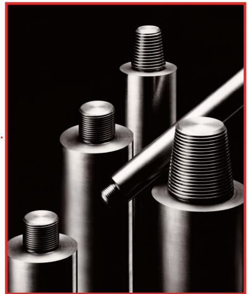
HC Starck uses the electron beam (EB) melting process to manufacture Moly melt EB glass melting electrodes. EB melting technology uses recycled molybdenum as its raw material, which is prepared by being 'bombarded' with electrons in the furnace. The material melts and falls into a water-cooled copper mould, where it solidifies into a round molybdenum ingot. The ingot is then forged and formed into the desired shape.
