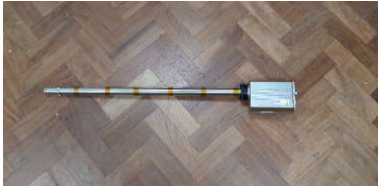
NIR-b-2k camera, 2ft probe, range 1000-1800C.
