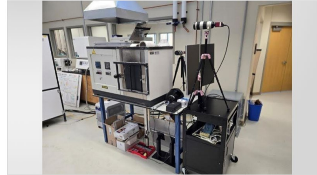
The cold-top furnace was set up at the University of Toledo, Ohio, USA.
