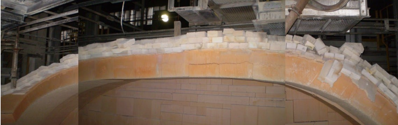
Overheating of fused cast AZS crown
